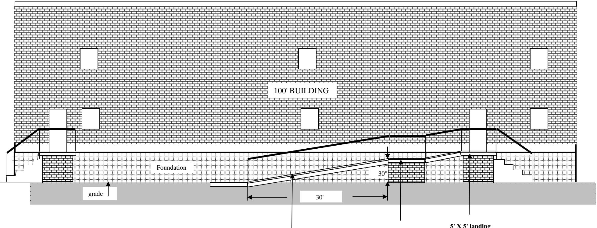
**Max. slope of ramp is 1' rise in 12' run. Easier slopes, to 1 in 20, are encouraged. Each 30" of rise requires a rest landing 5' long.**
